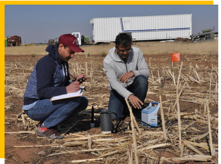
Rajan Ghimire (Right) demonstrating in-field CO 2 , soil moisture, temperature monitoring system to a graduate student, Vesh Thapa (left). Credit: Sangu Angadi
